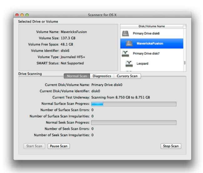
A surface scan test underway in Normal Mode
