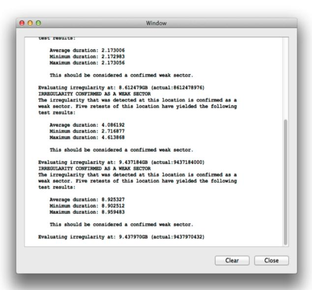
The Logging Window may be brought up in any tests to provide details about tests. In this screen capture, *Scannerz* is in *Diagnostics Mode* and evaluating a drive with some obvious problems.
