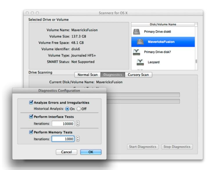
Diagnostics Mode tests may be configured to analyze errors and irregularities detected in previous tests, perform interface tests, and perform memory and system bus tests.
